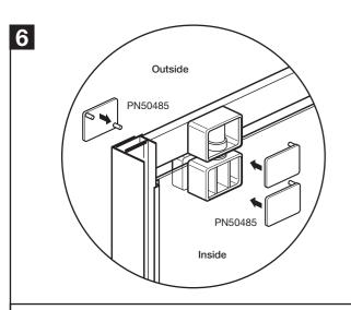
Push fit all 6 cover caps (PN50485) onto the pivot blocks at the top and bottom of the door (inside and outside).
