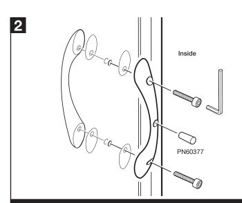
Fit the door handles to the doors with the allen bolts on the inside of the doors.
