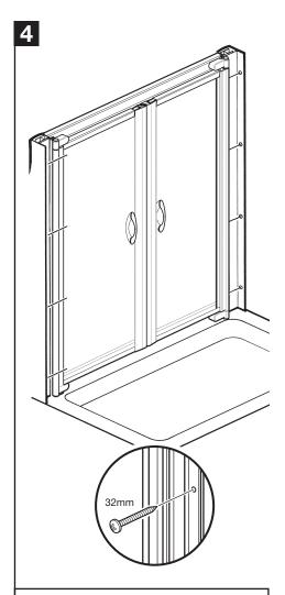
Place the door in position on the tray, fix the wall channels to the walls using 8  $\times$  32mm screws.
