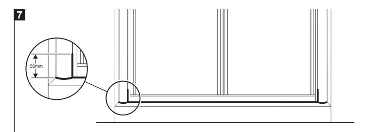
From the outside only, apply sealant to the bottom of the enclosure and 50mm up the wall channels as shown.
