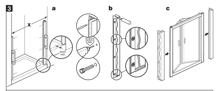
X = Door widths - 700 Door = 650 - 700mm ● 760 Door = 710 - 760mm ● 800 Door = 750 - 800mm ● 900 Door = 850 - 900mm
