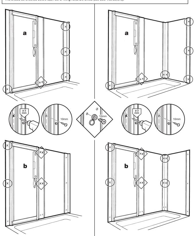
**a:** Check that the enclosure is perfectly vertical and sits evenly on the tray. Drill inside using a 3mm drill bit in the positions shown. Fix using 10mm screws. **IMPORTANT:** Screw caps are ONLY used on the 'inline joint post' (shown in the diamond shaped boxes).
