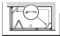
Only fit the wall bracket/s in the position/s shown (plan view of the enclosure).
