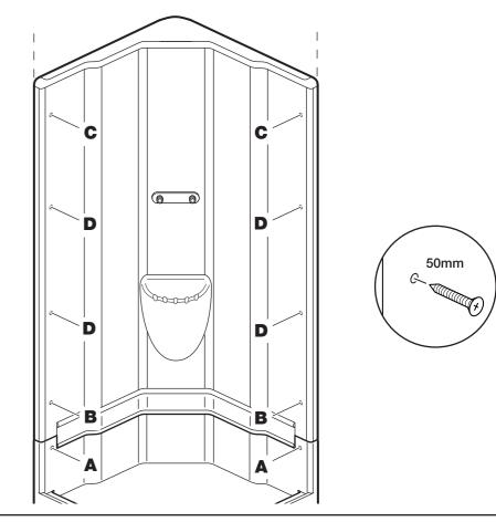
Reposition the pod back into lines marked on the walls. IMPORTANT: Fix in position DO NOT OVERTIGHTEN.
