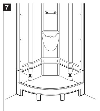
If after fixing the wall unit, there is a misalignment between the wall and base units, remove the two base unit fixing screws (X), realign the base and re-fix. **DO NOT OVERTIGHTEN.**
