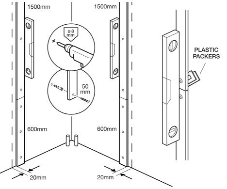
Using the short (600mm) and long (1500mm) battens, mark their positions on the side walls 20mm in from the marked lines. Drill through the battens in three positions into the wall using a 5mm drill bit. Remove the battens. Using a 8mm masonry drill bit open out holes in the wall. Insert wall plugs and fix the battens to the wall using 50mm screws. If the walls are not vertical use the plastic packers provided.
