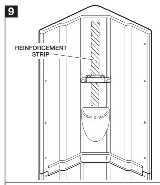
The shower handset riser rail should only be fitted onto the corner above the shower valve. The corner has built-in reinforcement for the fixing screws.
