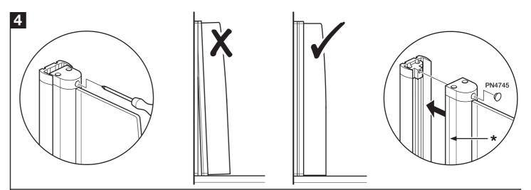
Adjust the curtain screen by tightening or loosening the top screw so that the bottom of the glass runs evenly along the bath rim. The curtain screen **MUST NOT** come out of the wall channel beyond the marked line (\*). Push fit the screw cap.
