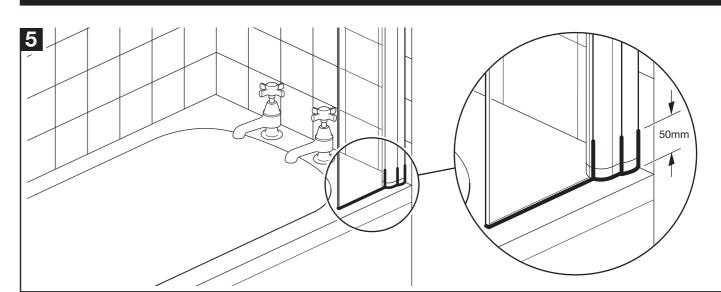
Apply silicone sealant to the outside of the curtain screen where shown.
