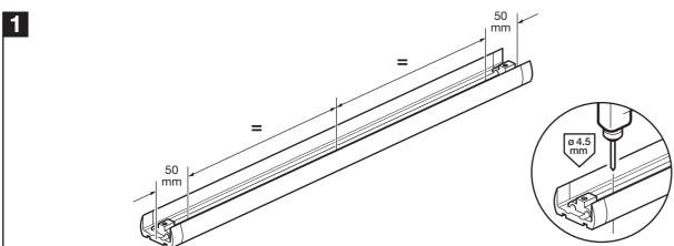
Drill three holes in the wall channel (PN80277) at points shown using a 4.5mm drill bit, through the grooved centre line.
