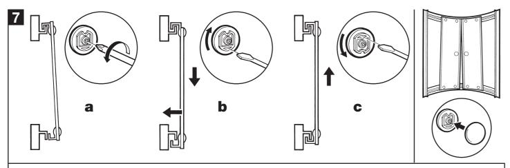
(a) Loosen top hanger screws (1 turn maximum) on doors. (b) Rotate top mouldings until bottom mouldings hook under bottom rail. (c) Rotate top mouldings to lift doors back up (with bottom sliders hooked under rail), re-tighten hanger screws. Doors may need adjusting (as in a, b & c) so they are square, meet in the middle and slide freely. Fit covers caps onto top and bottom mouldings.
