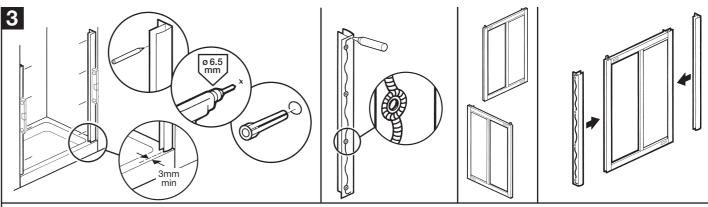
Place wall channels on the tray ensuring they are vertical and a minimum of 3mm back from the front of the tray. Place masking tape against the wall before marking the drill hole positions (this will prevent the drill bit slipping). Drill 6.5mm holes, 30mm deep and insert wall plugs.
