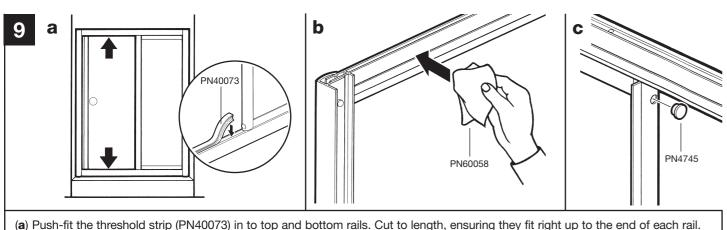
(b) Lubricate inner top and bottom rails with wipe provided. (c) Push fit the two hole plugs (PN4745) at the top and bottom of the fixed panel.
