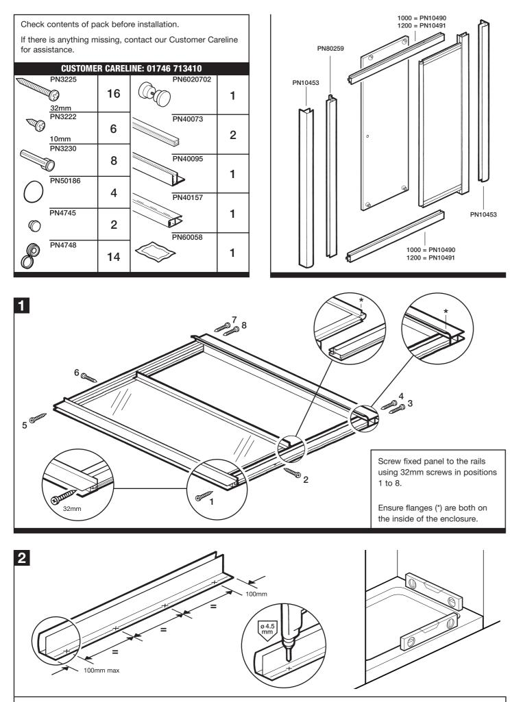
Drill holes in both wall channels (PN10453) at points shown using a 4.5mm drill bit, through the edge shown and in the grooves. Ensure shower tray is level in all directions.
