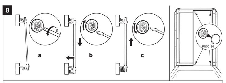
The door may need adjusting (as in a, b & c) so it is square, slides freely and the magnetic seals meet when the door is closed. (a) Loosen top hanger screws (1 turn maximum) on door. (b) Rotate top mouldings until bottom mouldings hook under bottom rail. (c) Rotate top mouldings to lift the door back up (with bottom sliders hooked under rail), re-tighten hanger screws. Fit covers caps onto top and bottom mouldings.
