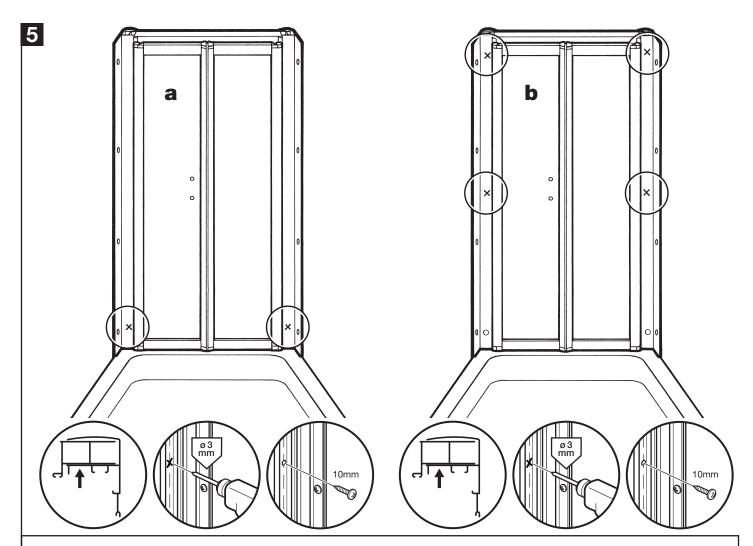
**a:** Check that the door is centrally positioned and perfectly vertical. Drill inside of the wall channels (in the groove) using a 3mm drill bit in the two lower positions shown. Fix using 2 x 10mm screws.
