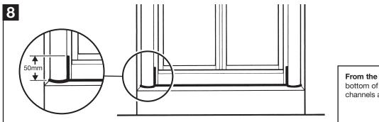
From the outside only, apply sealant to the bottom of the enclosure and 50mm up the wall channels as shown.
