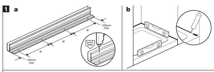
a: Drill holes in both wall channels at points shown (in the groove) using a 4.5mm drill bit.
