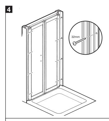
Place the door in position on the tray, fix the wall channels to the walls using 8 x 32mm screws.
