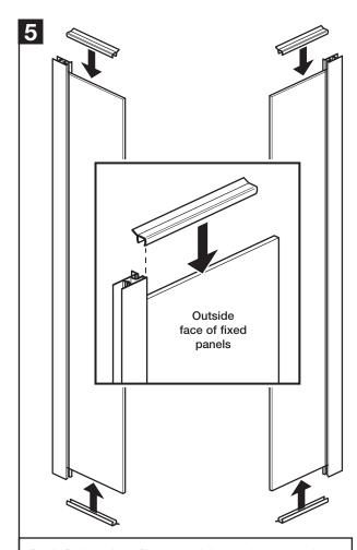
Push fit the 'short flipper seals' onto the top and bottom edges of both fixed panels - flush against the metal profile. **Ensure the flipper seal 'flaps' are on the inside of the fixed panels. Note:** Wetting the glass with water will help fit the seals.
