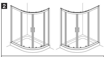
The Offset Quadrant can be assembled with the offset on either the right or left. **Note:** The following instructions show installation of the Quadrant.
