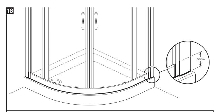
**From the outside only**, apply sealant to the bottom of the enclosure and 50mm up the wall channels and vertical joints as shown.
