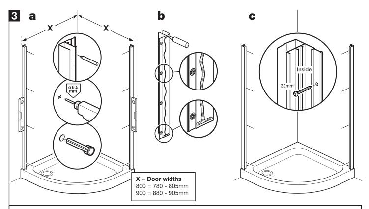
**a:** Place the wall channels on the tray ensuring they are vertical and an equal distance back from the front of the tray. Place masking tape against the wall before marking drill hole positions, this will help prevent the drill bit slipping. Drill 6.5mm holes, 30mm deep and insert the wall plugs. **b:** Apply sealant to the back of the wall channels and around the fixing holes.
