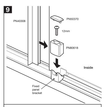
Fit 'flipper seals' (PN40308) onto the edge of the fixed panels. Ensure the flipper seal 'flaps' are on the inside.
