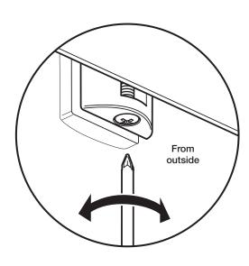
The 'wheels' at the top of the doors may need adjusting so that the doors slide freely and the magnetic seals meet evenly when the doors are closed.
