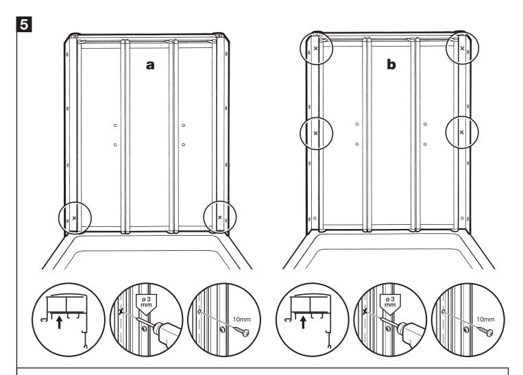
**a:** Check that the door is centrally positioned and perfectly vertical. Drill inside of the wall channels (in the groove) using a 3mm drill bit in the two lower positions shown. Fix using 2 x 10mm screws.
