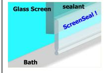
Apply sealant to serrated side of profile in continuous bead.
