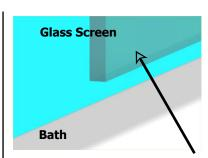
Clean along complete outer or inner screen with alcohol wipe.
