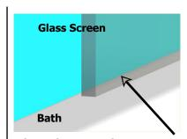
Clean along complete outer or inner screen with alcohol wipe.
