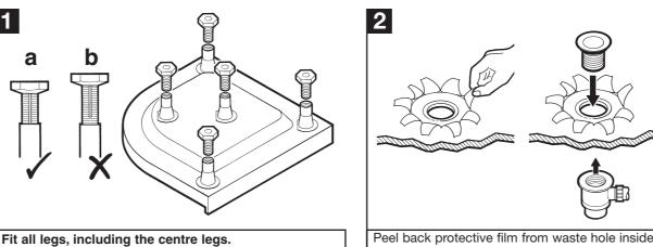
Peel back protective film from waste hole inside tray and fit waste outlet. Putty, mastics or acrylic sealant will damage the surface of the tray. Only use silicone sealant.
