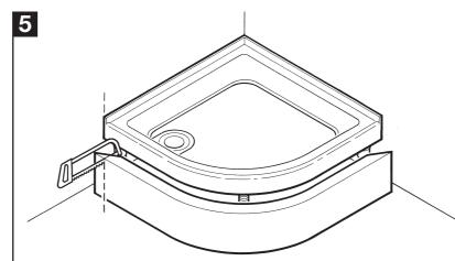
If necessary, carefully cut the outside edges of panel to fit.
