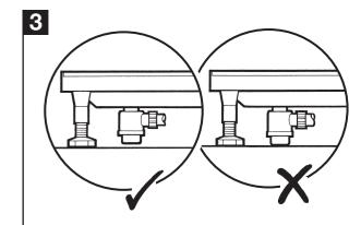
Place tray in position and fit waste pipe. Make sure pipe work is clear of floor, and base of tray.
