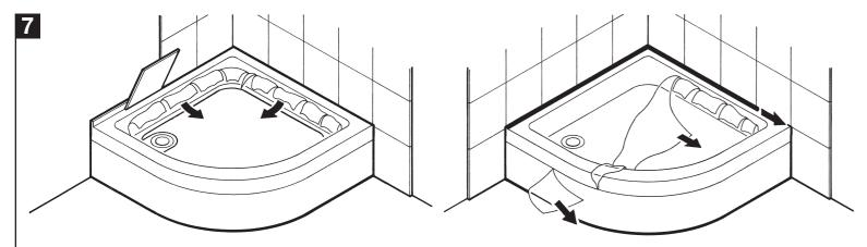
Peel back protective film from back edges of tray. Tile over upstands. Seal wall edges of tray with silicone sealant. Remove film from tray and panel, only remove cardboard tray protector when final installation of enclosure is complete.
