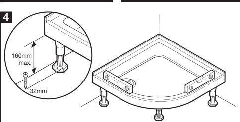
Adjust legs where necessary. Check tray is level in all directions (there is a built in fall on the tray for water drainage). **Centre legs MUST make contact with the floor.** Fix legs to the floor using 32mm screws, where accessible.
