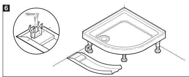
Align the panel up with the tray, fit brackets and mark centre line of brackets onto back of the panel. Ensure the direction arrow on the panel clips point upwards. Fix the brackets to the panel using 16mm screws. Push fit panel into place.
