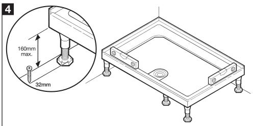
Adjust legs where necessary. Check tray is level in all directions (there is a built in fall on the tray for water drainage). **Centre legs MUST make contact with the floor.** Fix legs to the floor using 32mm screws, where accessible.
