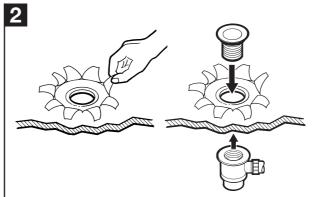
Peel back protective film from waste hole inside the tray and fit waste outlet. Putty, mastics or acrylic sealant will damage the surface of the tray. Only use silicone sealant.
