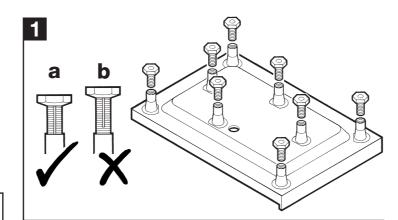
**Fit ALL legs, including the centre legs. Note:** The legs must be screwed in far enough that the end of the groove on the leg is **NOT** visible (a).
