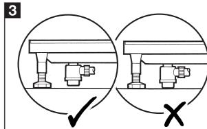
Place the tray in position and fit waste pipe.
