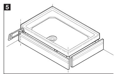
If necessary, carefully cut the outside edges of panel/s to fit.
