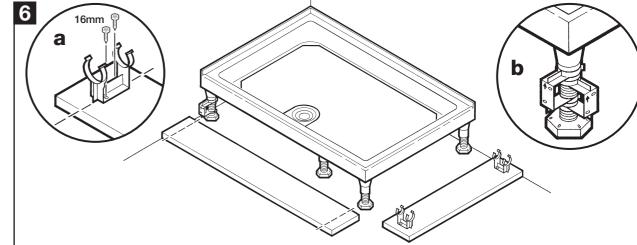
Align panel/s up with tray, fit brackets and mark centre line of brackets onto back of panel/s. Ensure the direction arrow on panel clips point up and fix to the panel/s using 16mm screws (a). **Corner leg:** Panel clips must be fitted to panel/s so they are staggered and do not clash with each other when fitted to legs (b). Push fit panel/s into place.
