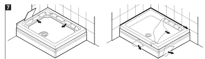
Peel back protective film from back edges of tray. **Tile over upstands. Seal wall edges of tray with silicone sealant.**When the final installation of the enclosure is complete, remove the cardboard tray protector and the remaining protective film.
