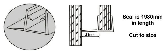
Important: Measure the thickness of your glass door plus the gap between your shower door / screen and the bath to ensure this seal will fit.
