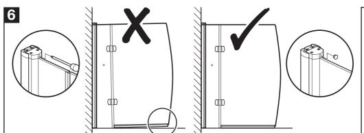
Adjust the bathscreen by tightening or loosening the screw at the top so that when opened, the bottom seal gently brushes the bath rim evenly along its length.
