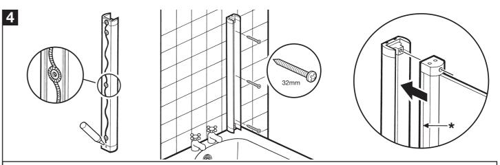
Apply silicone sealant to back of wall channel as shown. Fix wall channel to wall using the 32mm screws. Insert the bathscreen assembly into the wall channel fully tightening the top screw. The fixed panel **MUST** insert into the wall channel beyond the line marked (\*).
