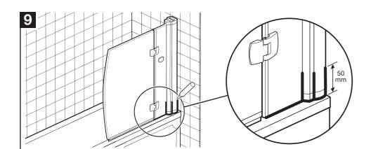
Apply silicone sealant to the outside of the fixed panel and bathscreen where shown.
