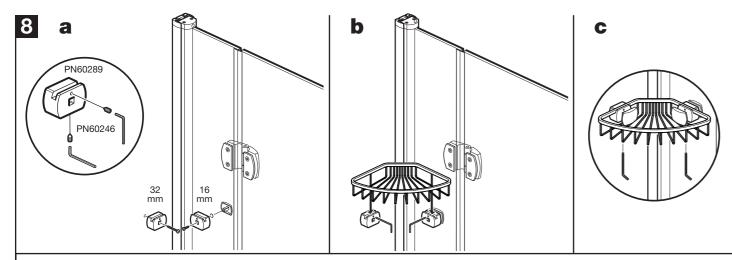
**a:** Partially insert grub screws into both brackets. Attach a bracket to the fixed panel, fixing through the bracket into a bracket cover using the 16mm screw, **do not over tighten**. Fix the remaining bracket to the wall using a 32mm screw, do not over tighten. **b:** Position the basket down onto the brackets and tighten the grub screws. **c:** Push on the bracket covers and tighten the grub screws from below.
