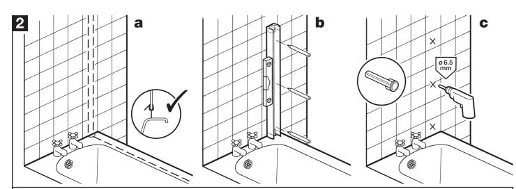
a: Position the fixed panel and bathscreen as far towards the inner edge of the bath as possible while being supported on the bath rim.
