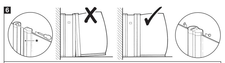
Insert the bathscreen into the fixed panel and tighten the top and bottom screws. The bathscreen MUST NOT come out of the fixed panel beyond the marked line (\*).
