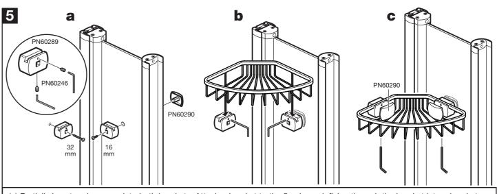
(a) Partially insert grub screws into both brackets. Attach a bracket to the fixed panel, fixing through the bracket into a bracket cover using the 16mm screw, do not over tighten. Fix the remaining bracket to the wall using a 32mm screw, do not over tighten. (b) Position the basket down onto the brackets and tighten the grub screws. (c) Push on the bracket covers and tighten the grub screws from below.
