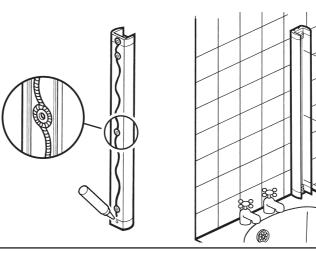
Apply silicone sealant to back of wall channel as shown.
