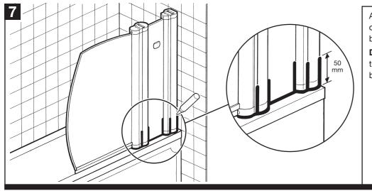
Apply silicone sealant to the outside of the fixed panel and bathscreen where shown.
