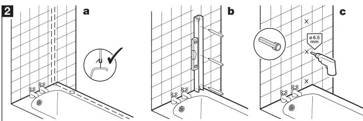
(a) Position the fixed panel and bathscreen as far towards the inner edge of the bath as possible while ensuring the vertical profiles are supported on the bath rim.
