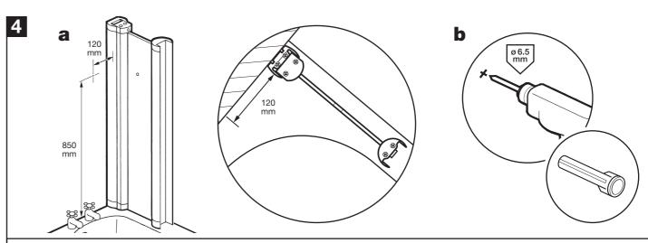
(a) Measure up 850mm from the top of the bath and 120mm in from the wall channel and mark the drill hole position onto the wall. Place masking tape against the wall before you mark hole position. (b) Drill a 6.5mm hole to a depth of 30mm. Insert wall plug.
