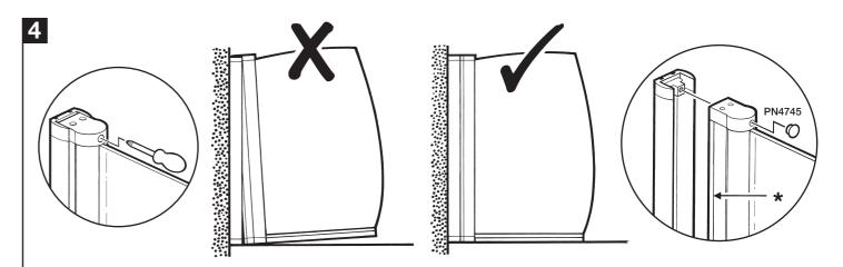
Adjust the bathscreen by tightening or loosening the screws (top and bottom) so that the bottom seal gently brushes the bath rim evenly along its length. **IF THE SEAL IS TOO TIGHT ON THE BATH THE BATHSCREEN MAY LEAK.**
