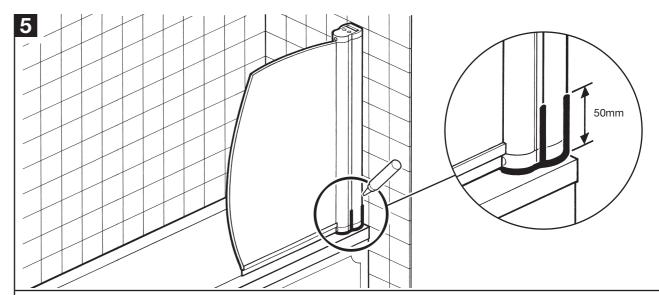
Apply silicone sealant to the outside of the bathscreen where shown.
