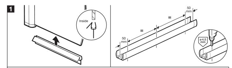
Fit the seal to the bottom of the bathscreen ensuring the seal 'flap' is on the inside of the screen, trim to length if required.
