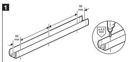
Drill three holes in the wall channel at points shown using a 4.5mm drill bit, through the grooved centre line.
