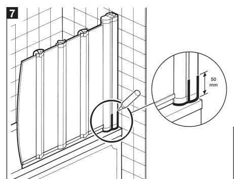
Apply silicone sealant to the outside of the screen where shown.
