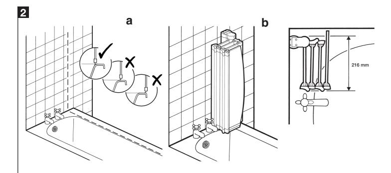
Position the screen so that it rests along the inner edge of the bath (a). It is advisable that the screen is fitted so that it will fold into the bath (b) Check the measurement above (4 and 5 panel version) to ensure you have sufficient space
