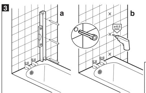
Position the wall channel, ensure it is perfectly vertical and mark off the drill hole positions against the wall (a). Place masking tape against the wall before you mark hole positions. Drill 6.5mm holes to a depth of 30mm. Insert wall plugs (b).
